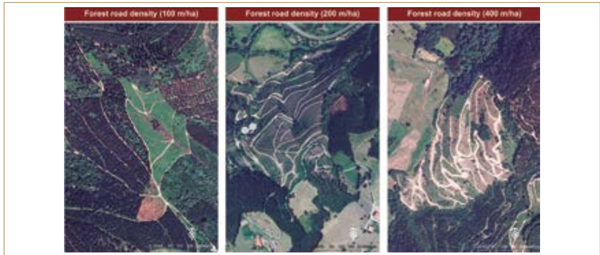
Figure 3. Density of forest roads in pine forest (left), eucalyptus forest (centre) and pine forests with inappropriate forest road networks (right).
