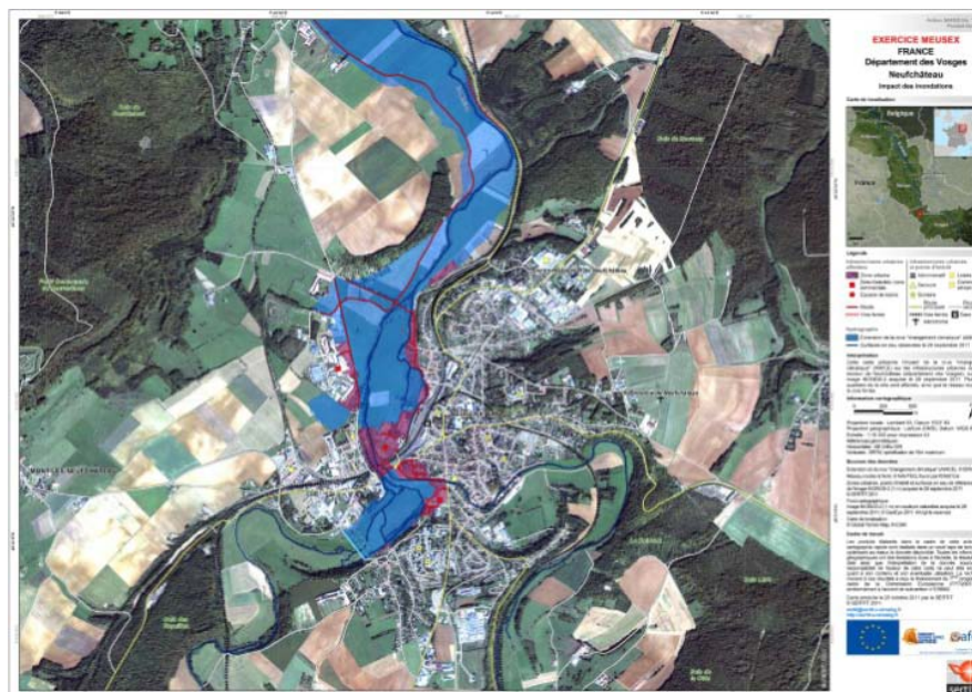
Figure 2: flood map obtained with SERTIT for the city of Neufchâteau (France); the blue zone corresponds to the flooded area, the red zone to the impacted urban area.
