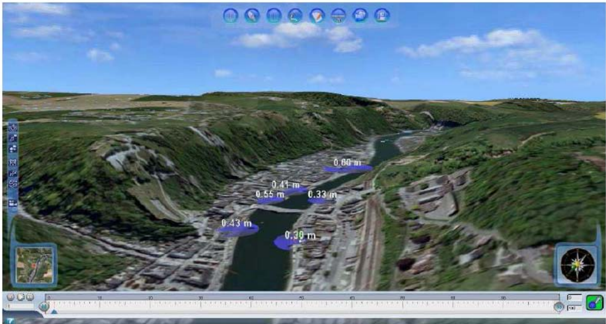
Figure 3: the “MobilAlarm” interface (APS - Belgium). The values which appear on the 3D simulator correspond to the water heights communicated by the citizens who are geolocated.
